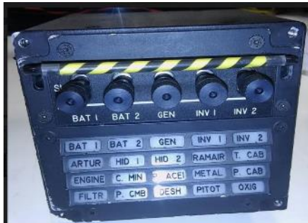
Panel de Alarma
